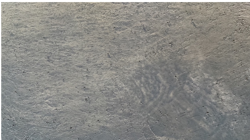
Fig. 87. Lawrence, R. (2022) 'Detail of marble and glue size surface with paint significantly thinned by mineral spirits'. [digital photograph].
