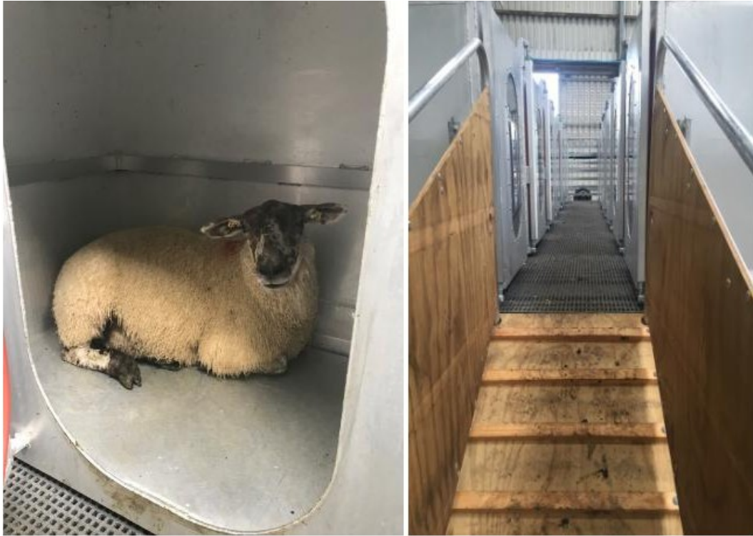
Figure 1.11: Portable accumulation chambers (PACs) used to measure methane emissions from sheep. Image sourced from (Teagasc, 2017)
