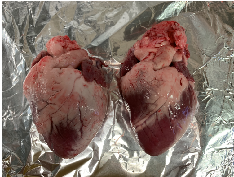
Figure 3.3: Two heart samples from A1 ( left ) and A2 ( right ). The hearts differ in size, shape, and amount of pericardial fat covering the epicardium. The pericardial fat extends around the whole heart, presenting a challenge when measuring the dielectric properties of the tissues on the exterior surface.
