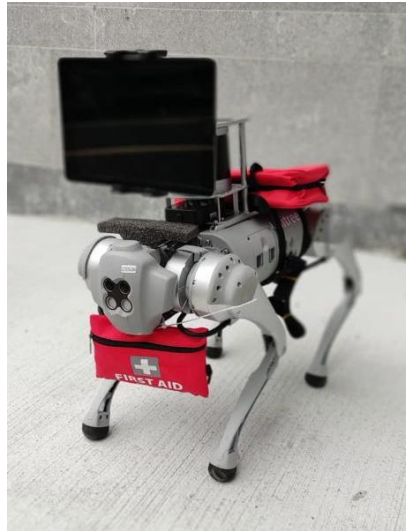
Figure 1: MADRA (Medical Autonomous Droid Remote Assistance) equipped with a medical kit.
