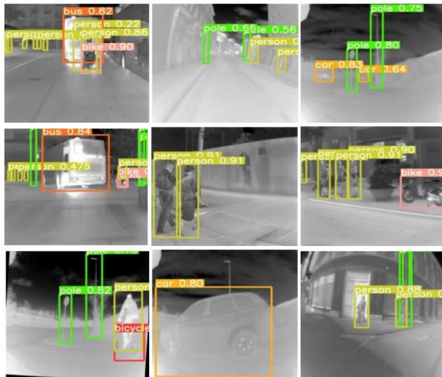
FIGURE 5. Inference results on nine different thermal frames using small, medium, large and x-large model variants of the Yolo v5 framework.
