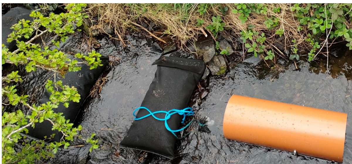
171 Figure 2. Schematic of different configurations of the intervention positioned in the stream. 172 The blue arrow indicates direction of water flow. Filter bags are upstream from the filter pipe. 173 Sampling points, colour-coded (see Section 2.4), are also indicated on the scheme. Photo shows 174 actual configurations in one of the streams, with first bag of three in the top left hand corner of 175 photo.
