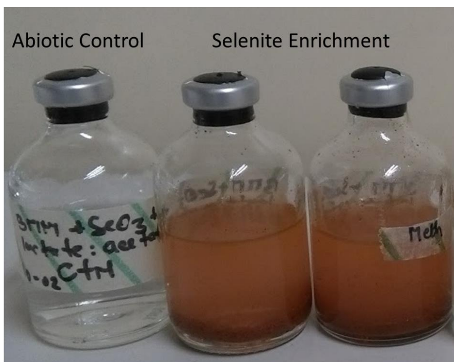
Figure 2. Selenium nanoparticle production in enrichment cultures and abiotic control containing no biomass.
